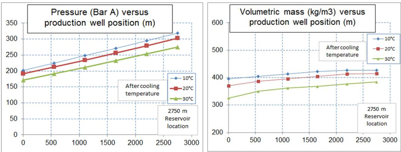
Figure 6.2.a and b – Pressure and volumetric mass along production well pipe for three cooling temperature values – Wellhead entrance.
