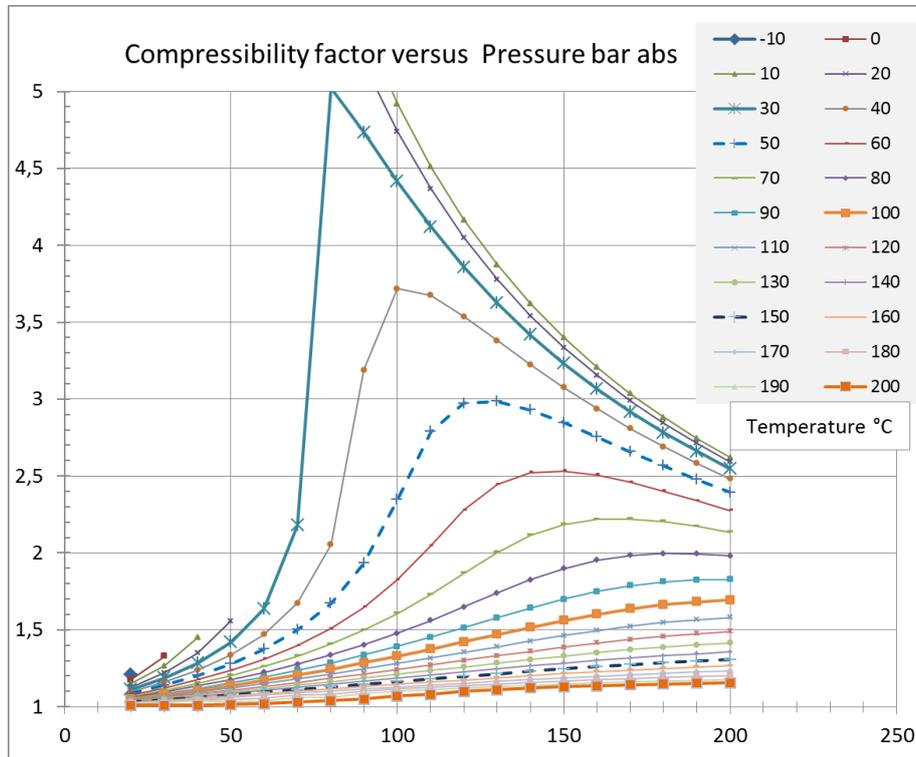
Figure A1 – Compressibility factor versus pressure (abscissa) and temperature
