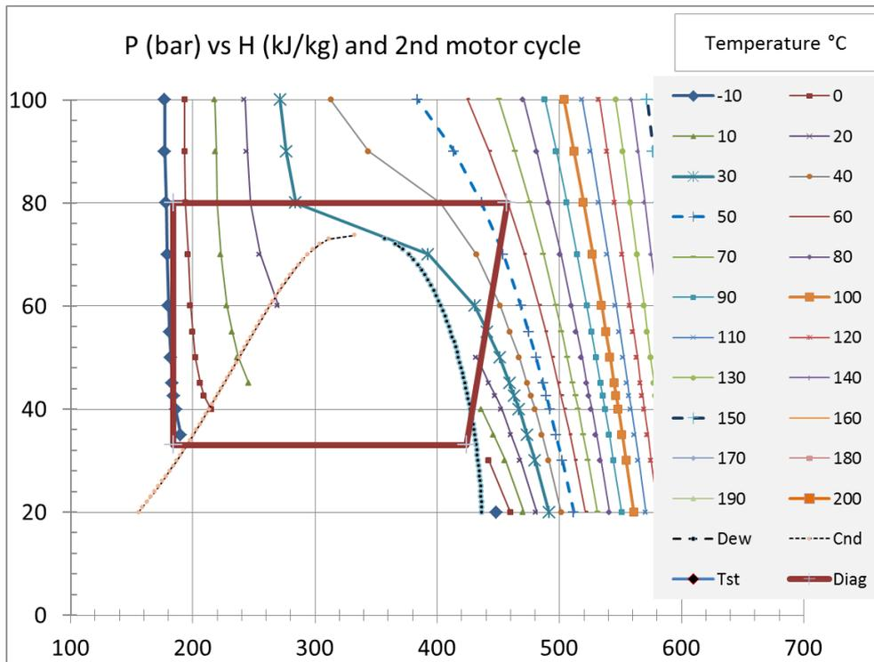
Figure 7.2 – Pressure – Enthalpy CO2 diagram with representation of the motor cycle operating with pure CO2. Cycle operation down to minus 6.8 °C.
