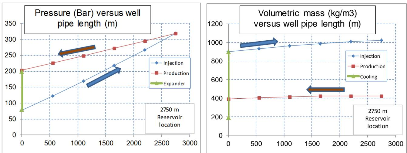
Figure 5.1.a and b – Pressure and volumetric mass along injection and production well pipes.
