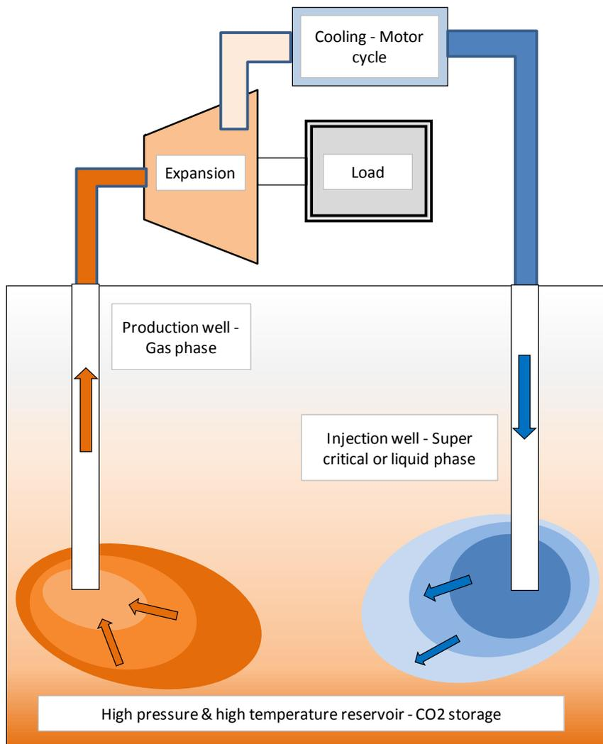
Figure 2 – Schematic of the carbon dioxide geothermal loop.
