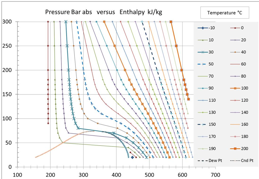
Figure A5 – Pressure versus enthalpy (abscissa) and temperature lines with dew and condensation lines
