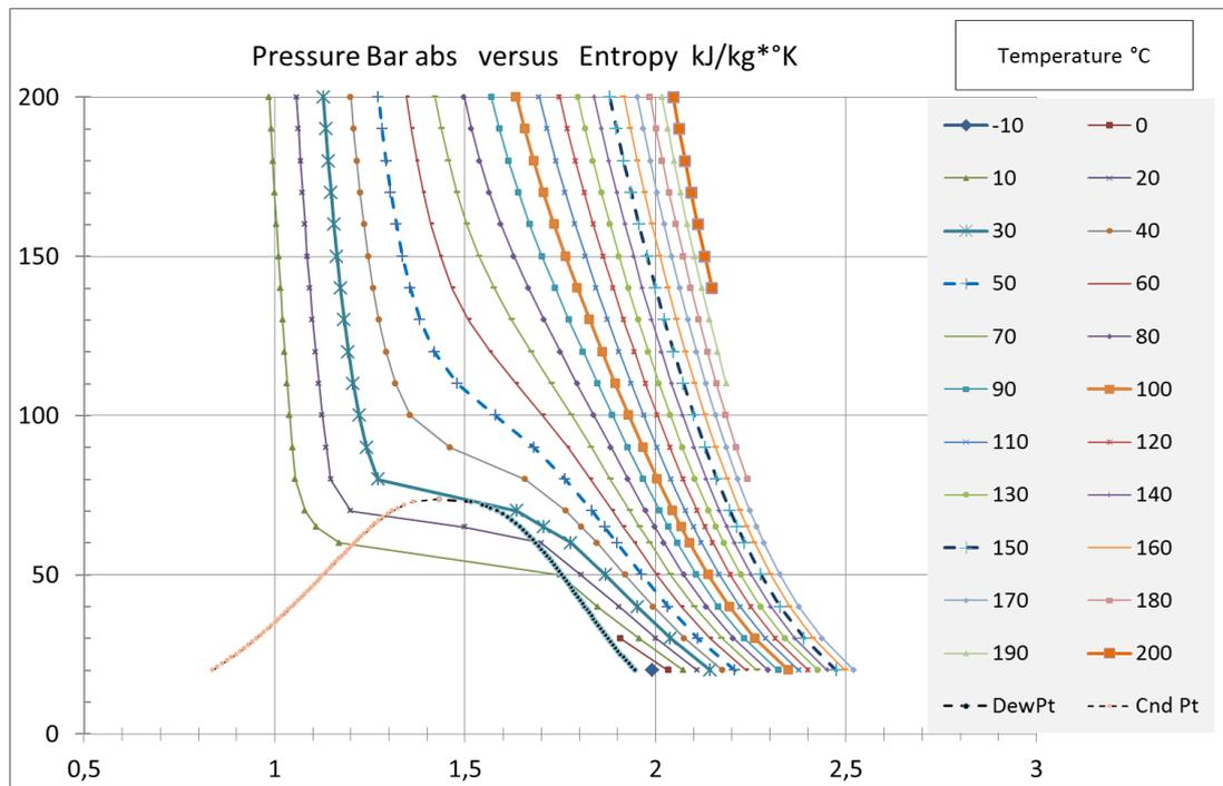
Figure A6 – Pressure versus entropy (abscissa) and temperature lines with dew and condensation lines
