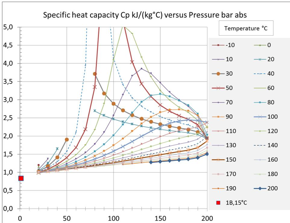
Figure A3 – Specific heat vs pressure (abscissa) and temperature – Square: 1 Bar abs; 15 °C
