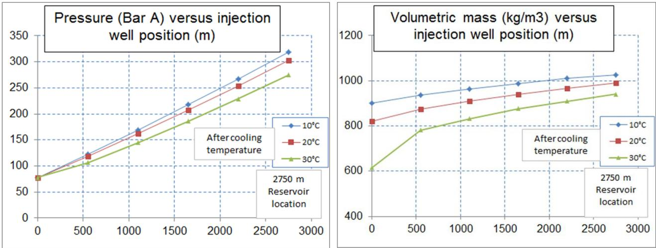
Figure 6.1.a and b – Pressure and volumetric mass along injection well pipe for three cooling temperature values at the wellhead.
