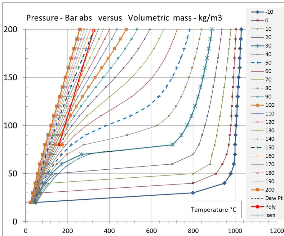
Figure A2 – Pressure versus volumetric mass (abscissa) and temperature
