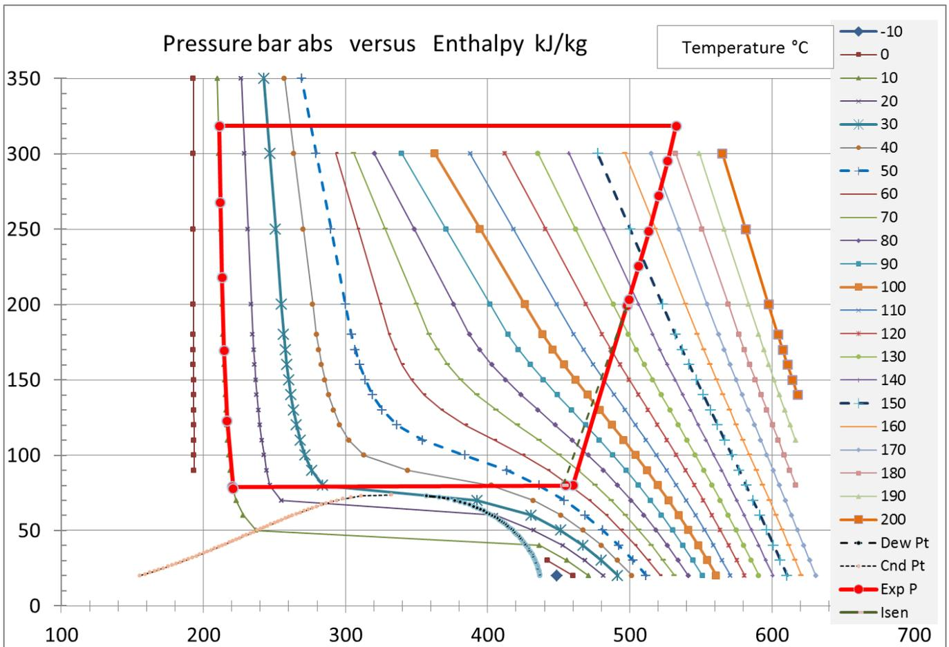
Figure 5.2 – Pressure versus enthalpy with temperature lines – Geothermal loop (In red) represented on a CO2 Mollier diagram
