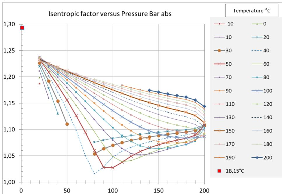
Figure A4 – Isentropic factor (indicative) vs pressure and temperature – Square: 1 Bar abs; 15 °C
