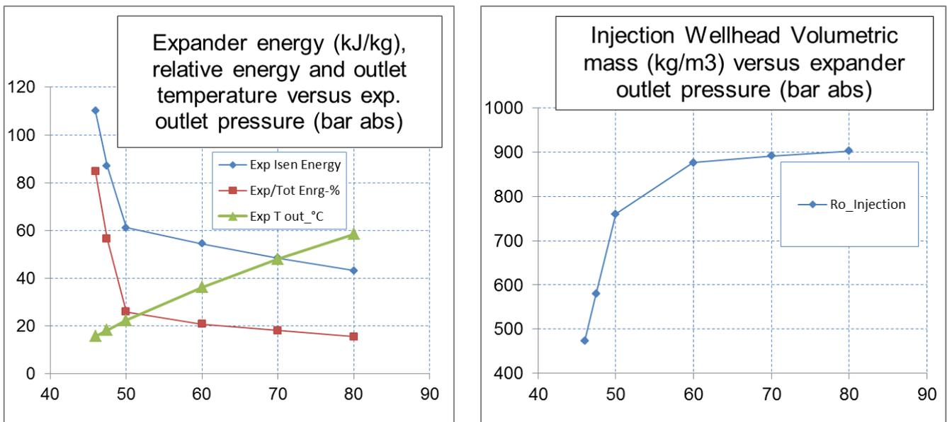
Figure 6.3.a and b – Expander isentropic energy and expander / total energy ratio (left); Injection wellhead volumetric mass (right) versus expander outlet pressure (Bar abs).
