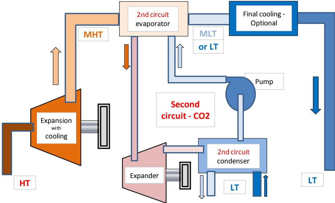
Figure 7.1 – Schematic of the secondary circuit for additional energy production.
