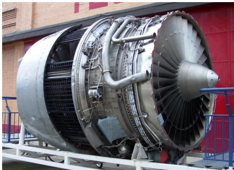
Figure 2 – Rolls-Royce RB211 Aero derivative gas turbine.
