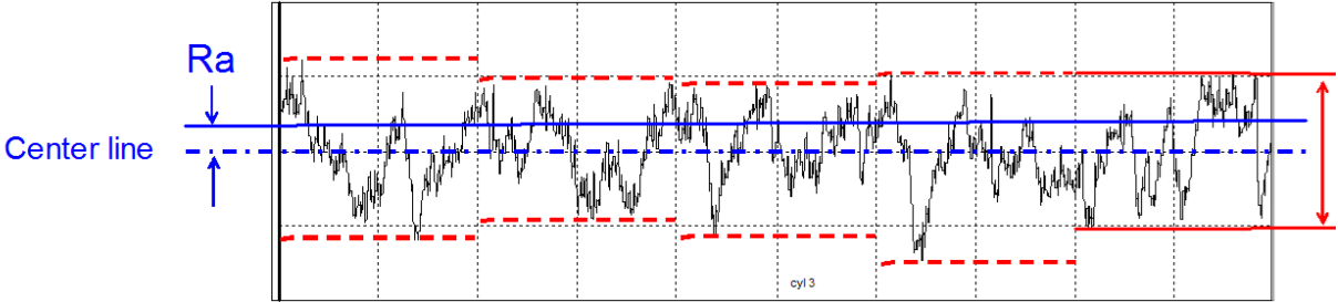
Figure 3 – Typical roughness profile with definition of the Ra and Rz parameters.
